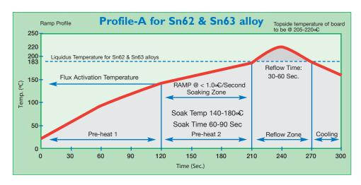
A profile utilizing a soak of up to two minutes at 155°C may help to minimize voiding in BGA assembles. This will allow more time for solvent components of the solder paste to outgas prior to reflow.
